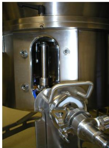
A VFC-300M shown with a 590L straight-sided Wurster insert. The Wurster system, as shown, includes the Wurster Accelerator spraying system, removable spray guns, and automatic partition height control.
