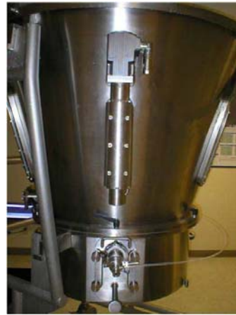
Stepper motors automatically control Wurster partition height.
