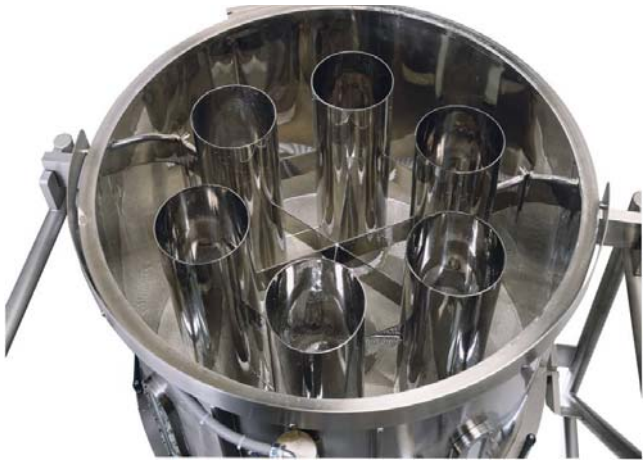
A six partition 590L Wurster insert with automatic control of partition height.
